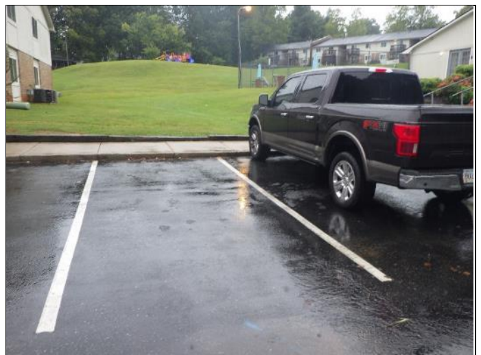
12. Parking near leasing office; note lack of Van-Accessible stall.
